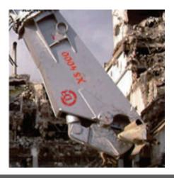
Weight:1250 kgsClosing force:1445 kNOpening jaw:350 mmPressure rating:350 barDepth jaw:410 mmFlow:100-160 lpm
