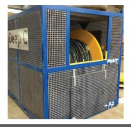
Dimensions (LxWxH): 2998mm x 2438mm x 2671mm Hydraulic output: Weight: 7 800 kgs
