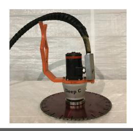
Dimensions (LxW):260x400 mmMax cutting disc:350mm/ 14"Weight:13 kgPressure rating210 barWeight in water:9 kgOptimum flow:50 l/min
