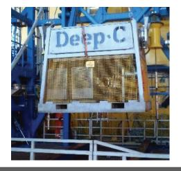
Dimension (LxWxH): 490 kW electrical 2700mm x 2100mm x 2600mm Available power: Weight: 3 200 kgs Control system: Project sepcific Weight in water: 2 500 kgs **Deployment:** 4,5 m Hs
