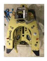
Dimension (LxWxH):1124x768x308 mmMax cutting size:450mm/ 18"Weight:35 kgPressure rating:175 barWeight in water:18 kgOptimum flow:50 l/min'
