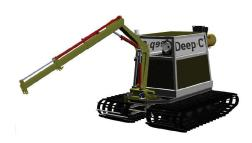
Outreach tooling: Outreach dredging: Swing on arm: 11,5 m 13-15 m 60 degrees Lift capacity: 900 kgs
