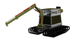
Outreach tooling: Outreach dredging: Swing on arm: 9 meters 11-13 meters 60 degrees Lift capacity: 900 kgs
