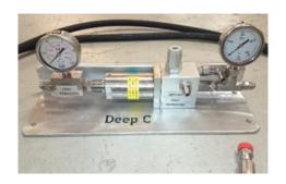
Dimension (LxWxH):400mm x 150mm x 150mmMax pressure inlet:200 barWeight (air):10 kgsMax flow:2,5 lpmMin pressure inlet:20 barIntensification ratio:4
