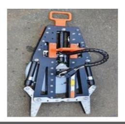
Dimension (LxW):1453 x 746mmMax cutting size:230mm/ 9"Weight:120 kgPressure rating:110 barWeight in water:90 kgOptimum flow:60 l/min
