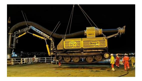
The Deep C SCV (Subsea Construction Vehicleis a poweful and versatile tracked subsea vehicle with unmatched 20" restricted dredging system. The Deep C SCV can perform several heavy duty tasks with subsea interchangeability, providing cost reductions on deck equipment, personnel and time.
